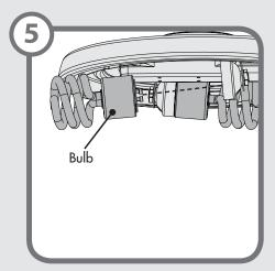
Install a light bulb in each socket.
